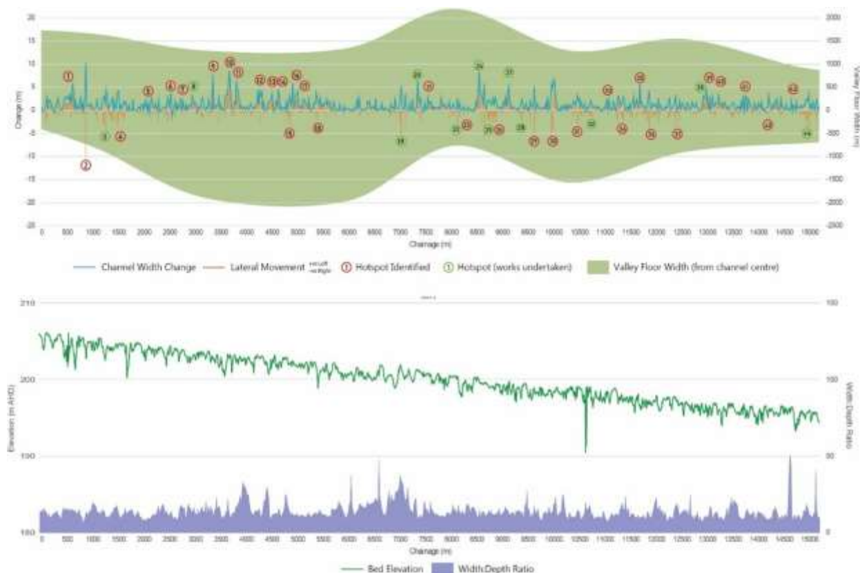
Figure 7 An example of a channel change diagram from the Mitta Mitta project integrated with long section and width to depth ratio
