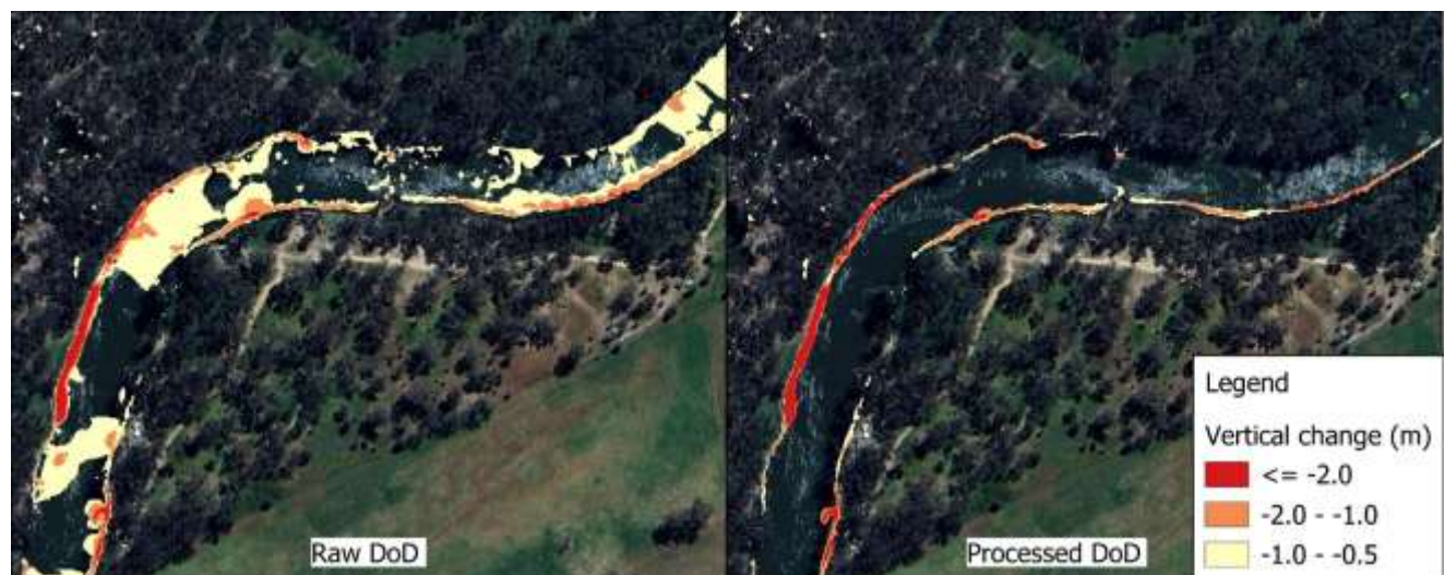
Figure 1 Example of a raw DoD showing errors associated with water surface and a processed DoD to reduce LiDAR error
