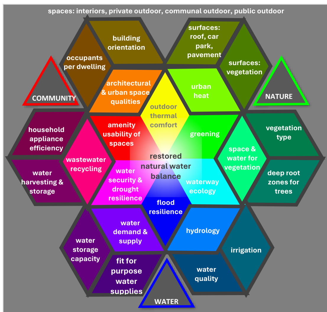
Figure 1 Additive RGB colour-coding framework developed for integrated waterway management in the Norman Creek study. Red represents community, green represents nature, and blue
