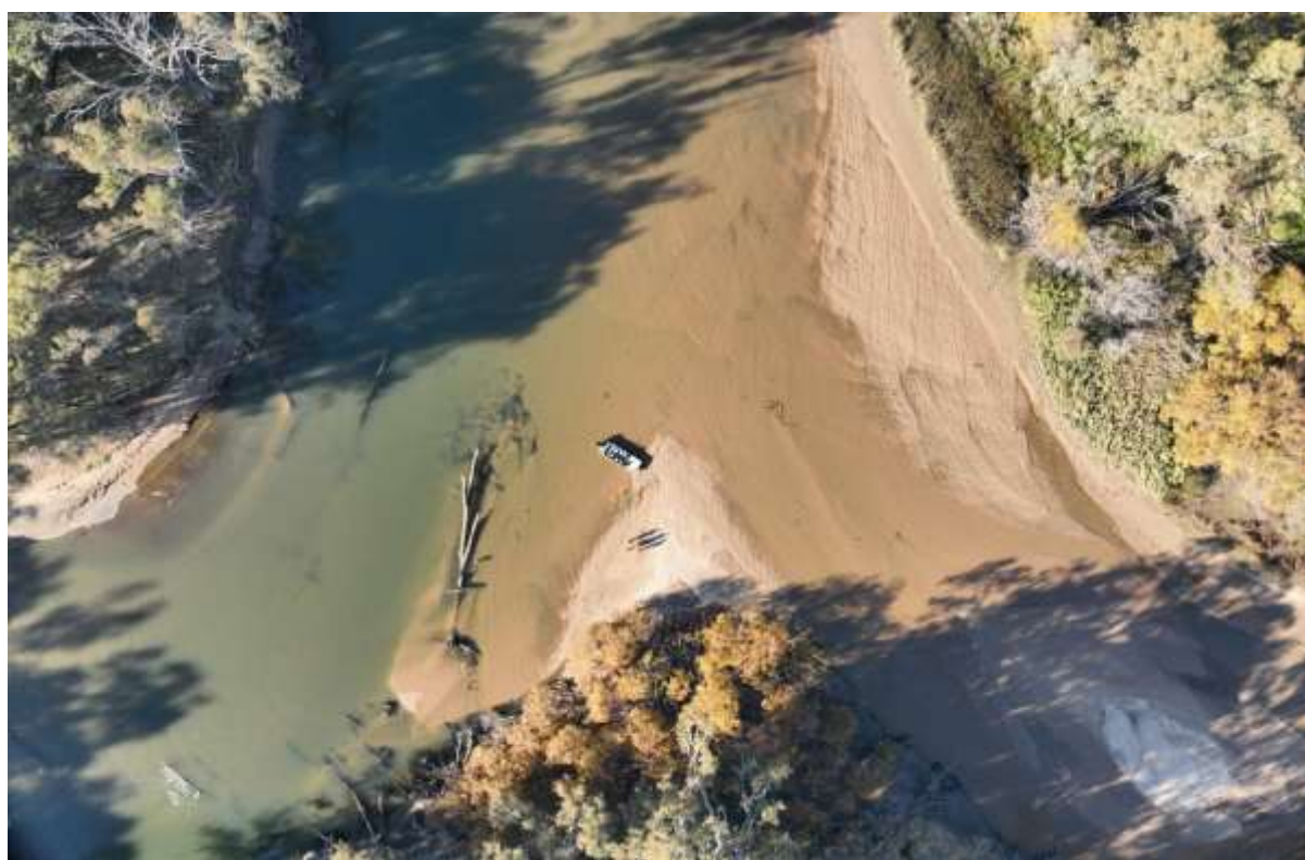
Figure 1 Photograph illustrating flow capture by Hans Creek (left) and infilling of the Murray River channel (right), demonstrating the need to define the “main channel” by hydraulic/geomorphic dominance rather than mapped labels
