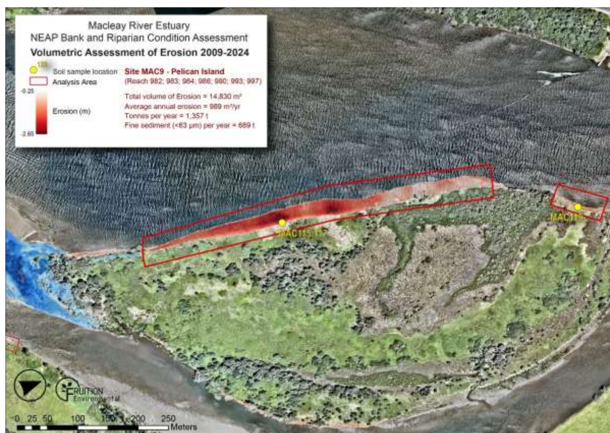
Figure 2 Geomorphic change along Pelican Island on the Macleay River estuary. Note that the erosion is mostly occurring as lateral scour, resulting in channel expansion. The GCD analysis cannot assess sub-tidal erosion volumes as no return points provide elevation or bathymetry data at the location
