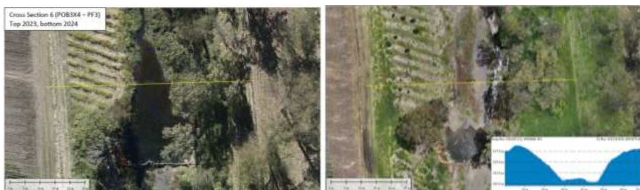
Figure 3 2023 and 2024 comparison of revegetation at a cross channel pilefield, showing development of an upstream bench and riparian vegetation strengthening (Parker et al., 2024) a) 2023 b) 2024. (Parker et al, 2024)
