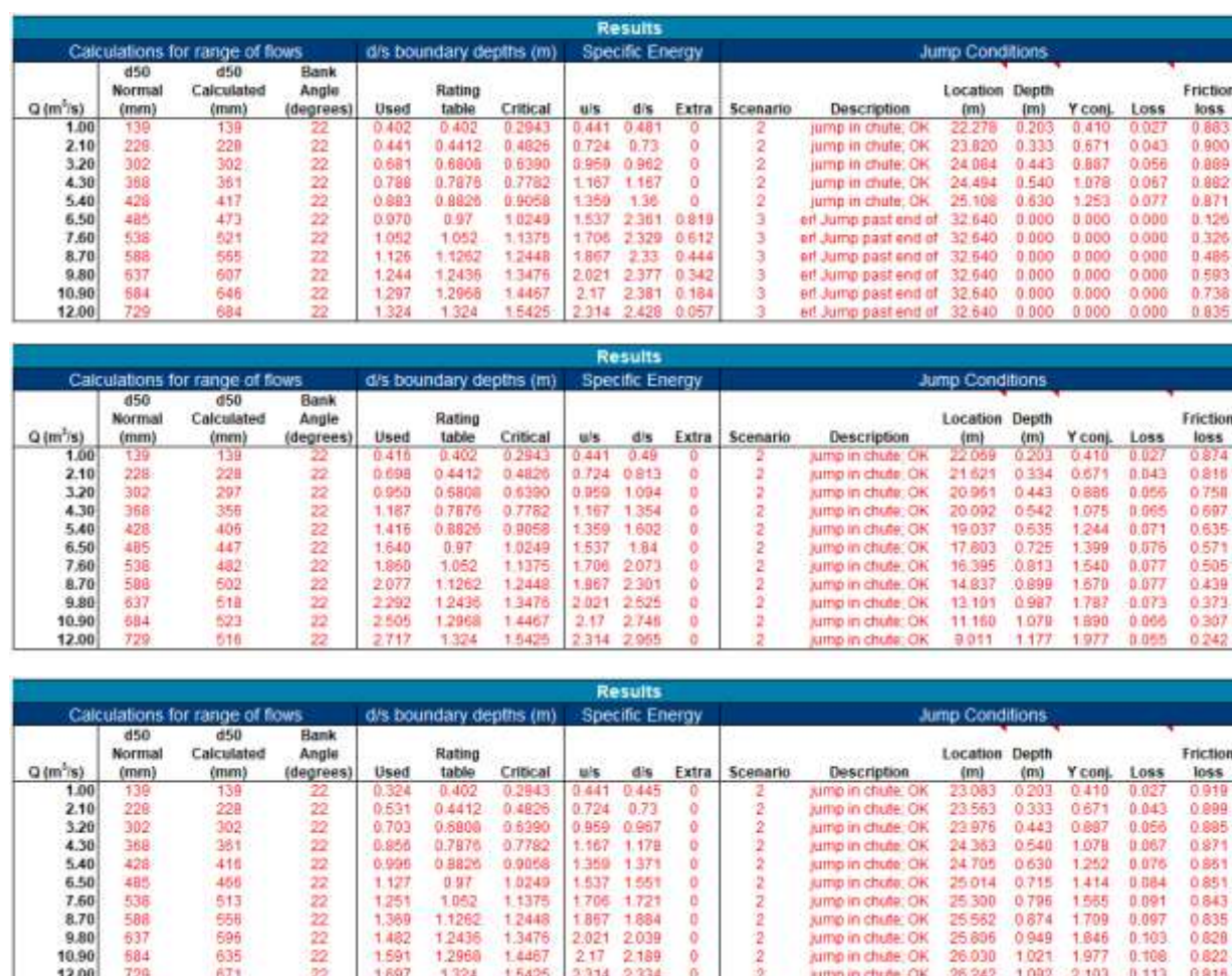
Figure 4 CHUTE results for Warrenheip Creek with boundary conditions of rating table (top), normal depth (middle) and critical depth (bottom)
