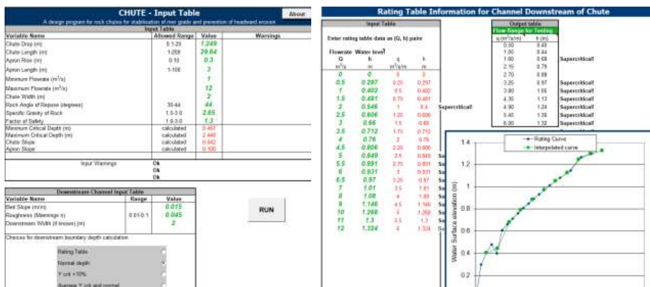
Figure 3 CHUTE input parameters (left), the rating table downstream of the chute from TUFLOW
