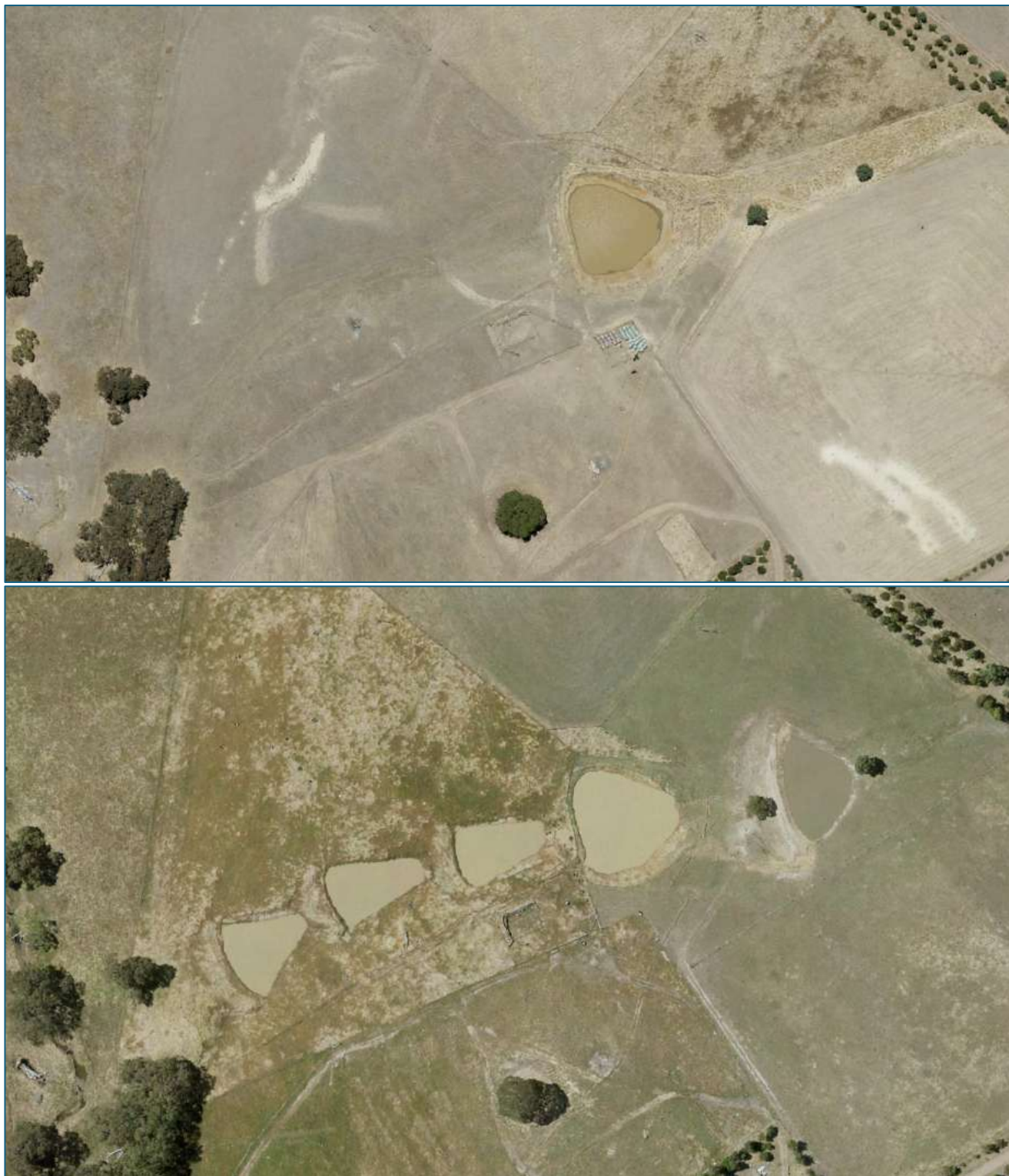
Figure 1 Change detection imagery showing the appearance of unauthorised dams between 2021 (top) and 2024 (bottom) (Source: ImageMapSA)
