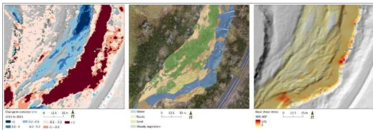
Figure 3 Monitoring datasets used in the Cann River (left) DEMs of difference, (middle) mapping of vegetation change, (right) modelled shear stress (40 % AEP) (Alluvium, 2024)
