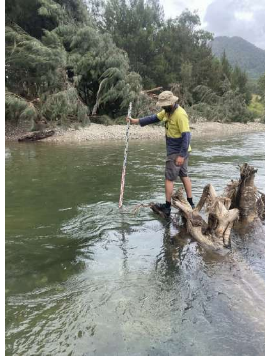
Figure 6 Scour from installed log after flood, ~ 1.4m deep, Five Day Creek, Comara, May 2025
