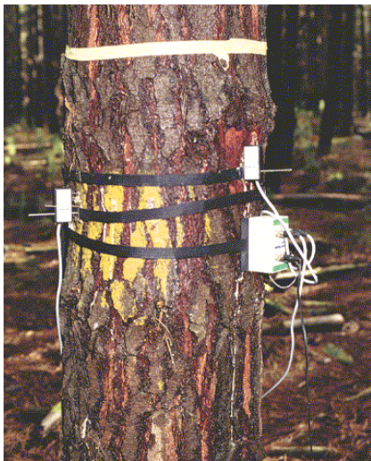
Figure 1: Heat pulse equipment attached to a tree at the site of the experiment.
