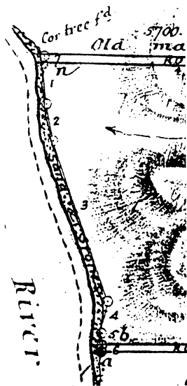
Figure 6: An 1887 resurvey of a portion of land at Lanyon ACT which a change in location of the bank of the Murrumbidgee River since the original survey. The strip of "sand and gravel" corroborates anecdotal material on changes to the river that occurred on and after a major flood of 1852.
