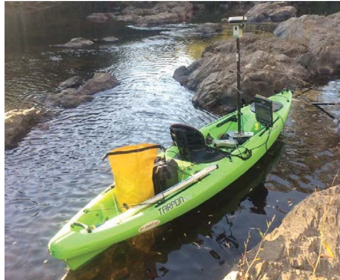
Figure 2. Kayak mounted bathymetric survey rig.
