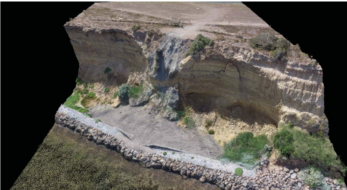
Figure 8. Aerial survey point cloud of an actively eroding cliff to monitor movement
