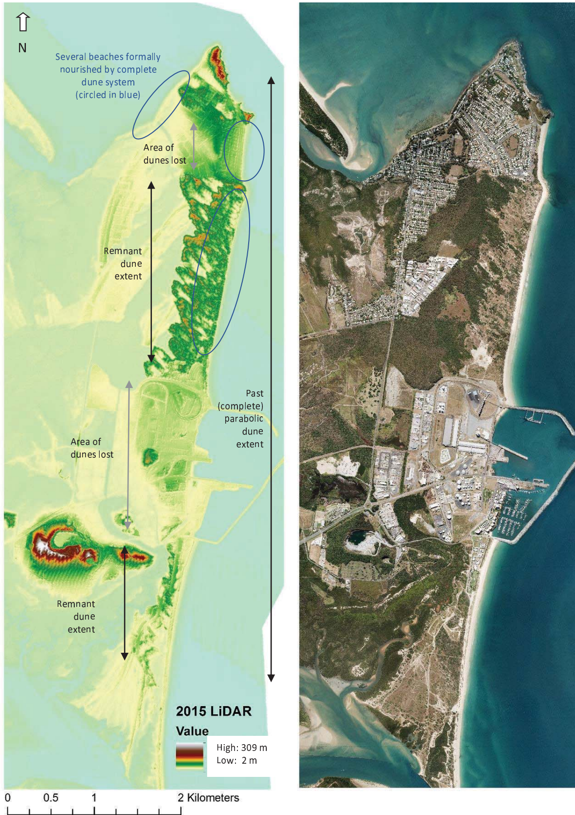
Figure 3. Slade Bay to Harbour Beach South – 2015 aerial and LiDAR imagery (DEHP 2015), presence of parabolic dune system evident from the LiDAR, with a loss of dunes at Lambert’s beach and at the harbour. Beaches formally nourished by the past (complete) dune system, via aeolian, cross-shore and long-shore transport processes, circled in blue.
