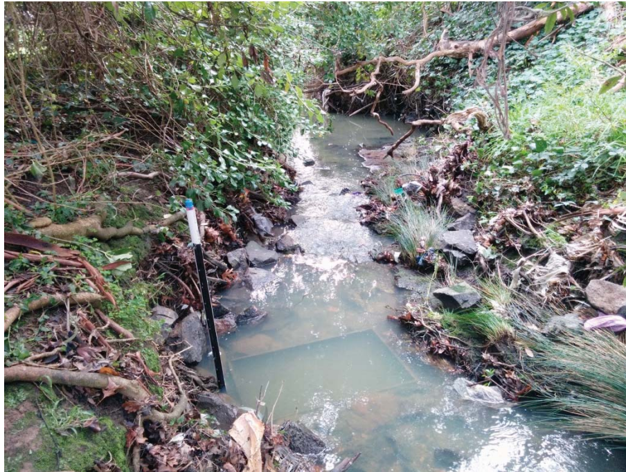
Figure 1. Forest Hill sediment trap, showing typical sampling setup
